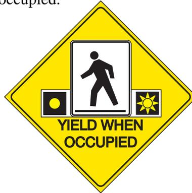
Special crosswalks on some curved streets have a **flashing yellow beacon** placed in advance to warn drivers that a pedestrian has pushed the button to cross the street.
