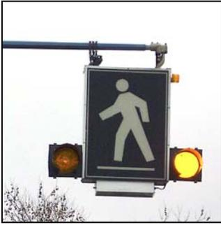
A special crosswalk is a traffic control device with pedestrian-activated overhead flashing yellow lights and downward lighting designed to do two things:
